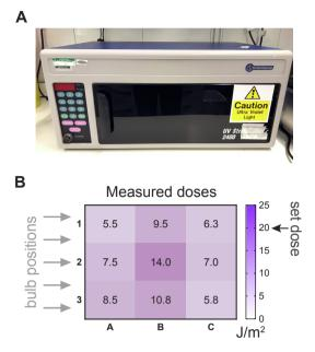
**Fig. 1.** Equipment for UV irradiation of cells. (A) A typical UV crosslinker (Stratalinker) device. (B) Variability of exposure across a typical UV crosslinker (Stratalinker) surface. Desired doses were set to  $20 \text{ J/m}^2$  UVC and actual emitted doses were measured with a UV meter at 9 different areas of the crosslinker surface. The average of four measurements is indicated. The positions of the device's light bulbs are indicated by arrows.
